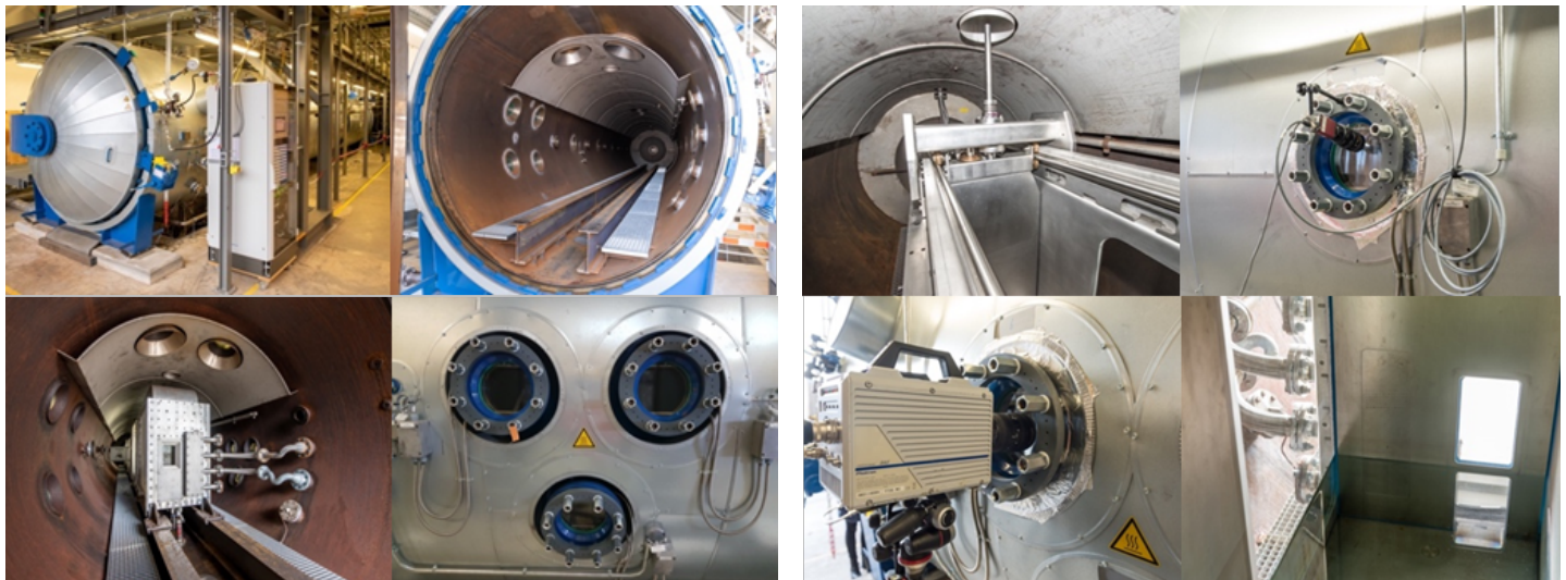
Figure 1. (top left panel) The Atmosphere (ATM) facility - (top right panel) The autoclave of the ATM - (bottom left panel) The flume inside the autoclave. At the fore front is the impact wall with its window - (bottom right panel) Three observation windows which are close to the impact wall.
